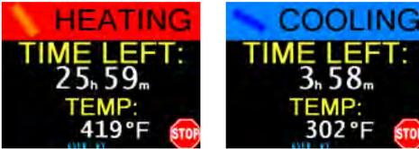
**TIME LEFT:** The total remaining time for the entire cycle, includes heating and cooling time.
