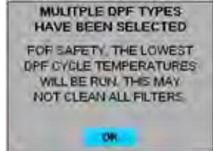
The GENERAL CLEANING CYCLE will heat to the temperature requirements set by the DPF manufactures. At the bottom of the screen the system will display the cycle which is chosen and the time of the cycle. If you wish to change the combination of filters in the Filtertherm<sup>®</sup> so a different cycle is run, you may press the back button to return to the filter selection. You can then remove the loaded filters, unselect them and select the new combination.
